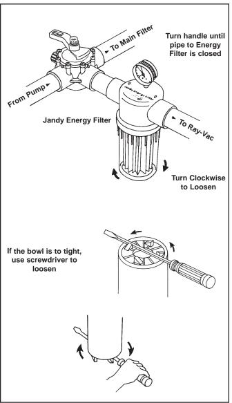
Figure 10. Removing Energy Filter
